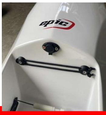
Photo 13. V-Series – footwell bungee and drain plug/breather tube in closed position
