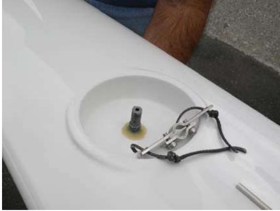
Photo 5. V-Series – run rudder post up through rudder housing in hull of boat
