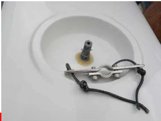
Photo 7. V-Series – center rudder pin in rudder post
