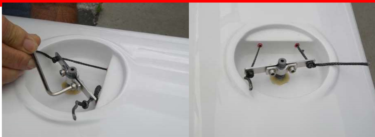
Photo 9. V-Series – once spreader bar is over the top of the rudder post, use allen wrench to tighten the spreader bar bolts so that top of rudder post and pin ends are pinched and held fast
