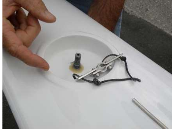
Photo 5. V-Series – run rudder post up through rudder housing in hull of boat
