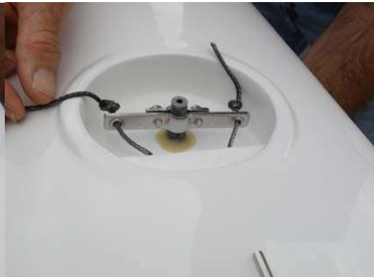
Photo 7. V-Series – center rudder pin in rudder post
